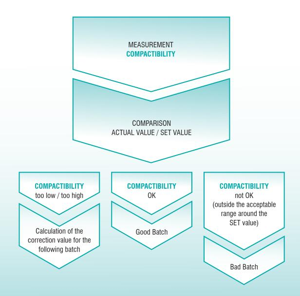
Adjustment of the amount of water to be dosed for the next batch by changing the target moisture value (see function graph).
