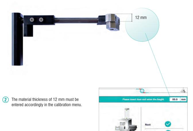
The 0% position must then be calibrated according to the software instructions.
