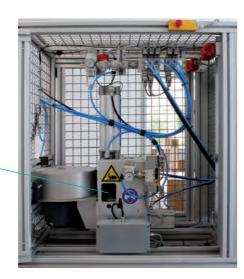
2 By actuating the release in the direction of the arrow, the test mandrel slips onto the base plate.
